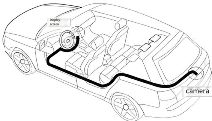
The rear-view camera provides a clear rear image through the connected terminal, which can detect and avoid blind spots and obstacles when reversing, reduce the risk of collision, and further improve the accuracy and safety of operation.
