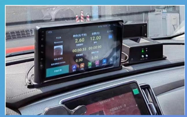
One of the simplest ways to install the taxi terminal is by placing it on the dashboard of your vehicle
